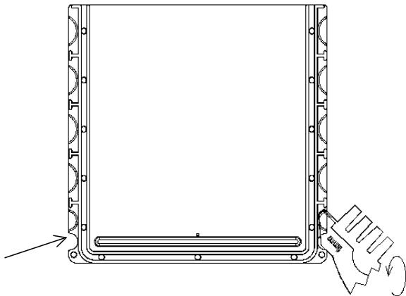
**Step 2:** After the sides are open, place the comb's slanted edge at a 45-degree angle between the plates at each bottom corner and twist firmly.
