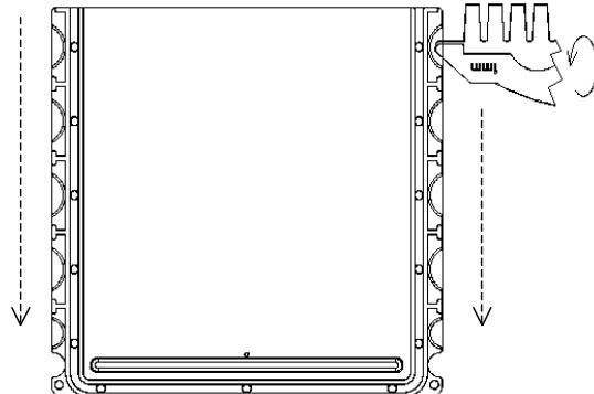
**Step 1:** Crack open cassette sides by inserting the comb tip into each of the notches around the cassette and twisting firmly. Starting with the notches at the top, move down each side of the cassette.
