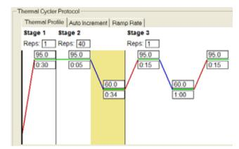
Stage 1: Initial denaturation Reps: 1  $95^{\circ}$ C 30 sec Stage 2: PCR Reps: 40  $95^{\circ}$ C 5 sec  $60^{\circ}$ C 30 - 34 sec \* Dissociation stage
